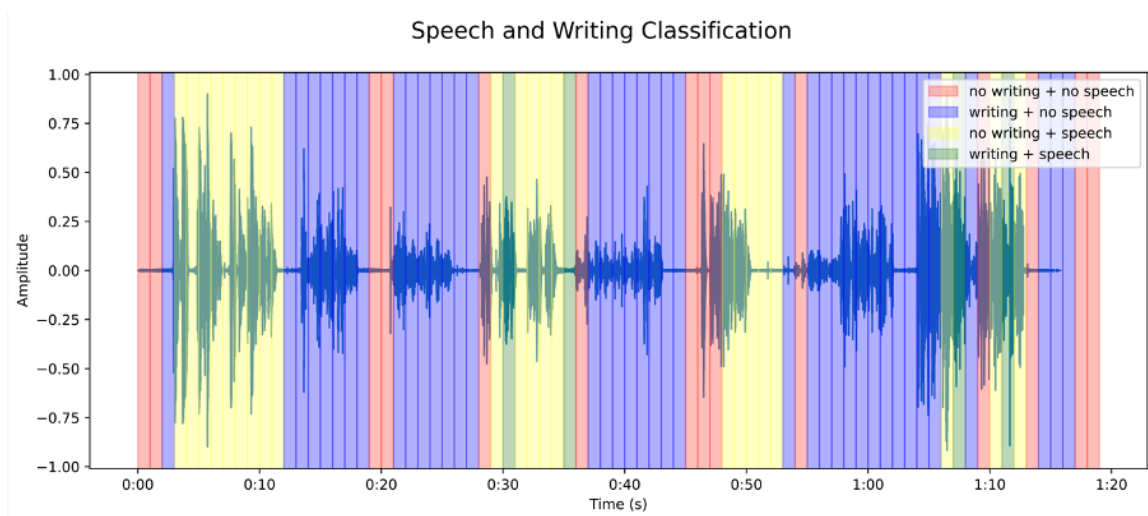
Figure 6.3: Classifier prediction combined with YAMNet speech prediction on mixed test data
