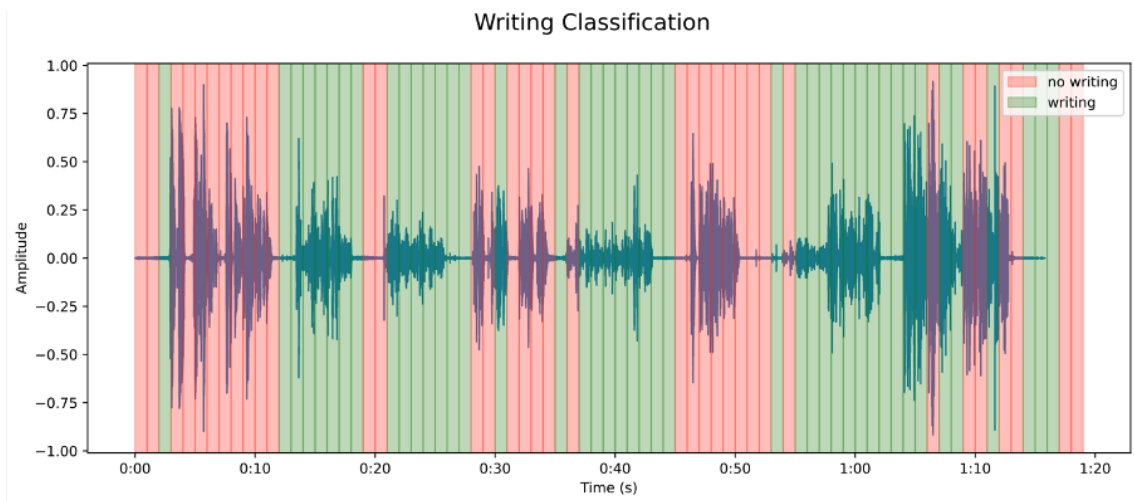
Figure 6.2: Classifier prediction for writing and no writing on mixed test data
